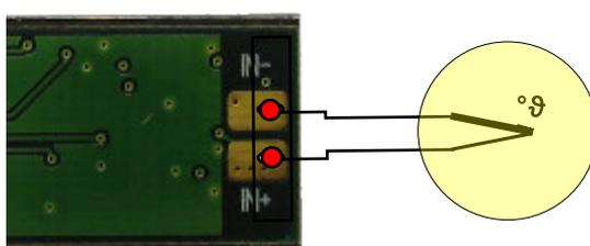
Use of isolated and also non-isolated thermocouples is possible
