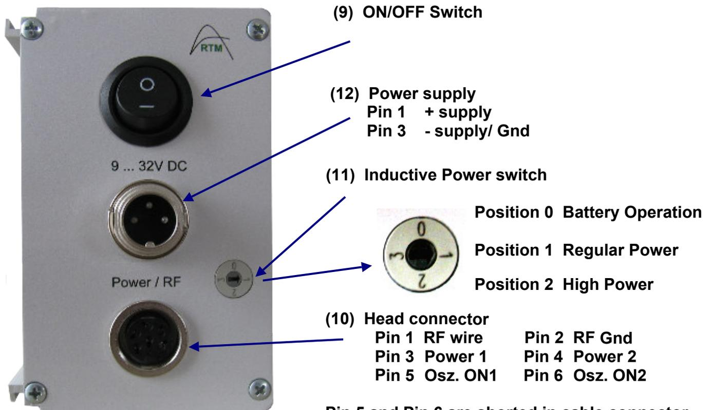
Pin 5 and Pin 6 are shorted in cable connector
