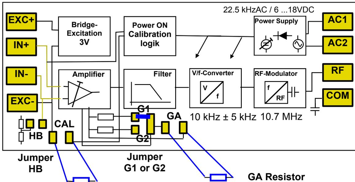
Possibilities installation of GA Resistor
