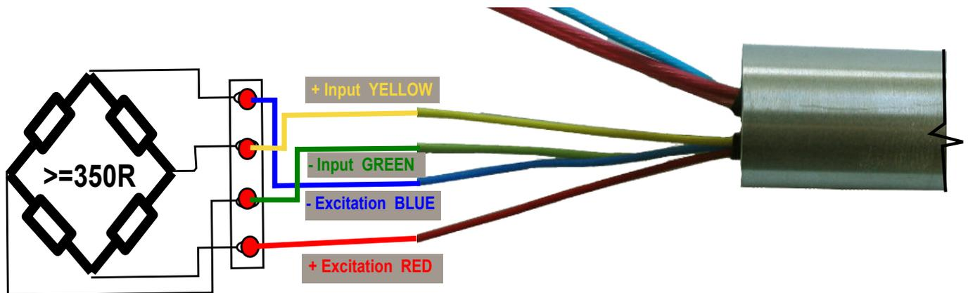
The calculation and installation of the Gain resistor and the Shunt occurs before imbedding in the cylindrical housing.
