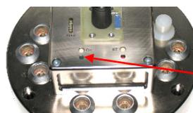
power on the mobile unit is done by pressing the key "On" and is showed by the green LED
