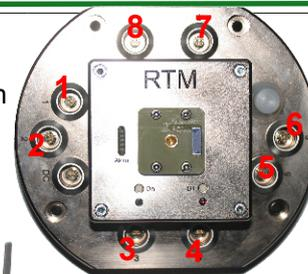
Connect the power cable with the socket " 8... 32VDC " of the reproducer and connect the colored plugs with a DC source
